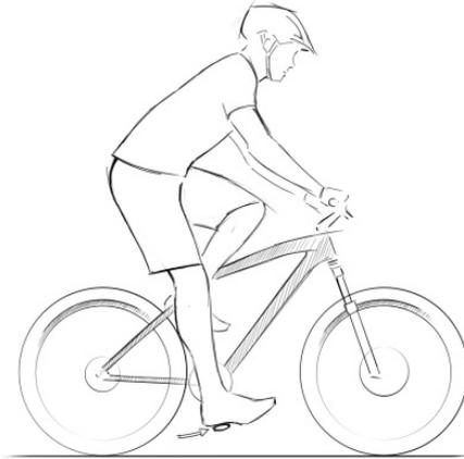
You should also adjust the saddle angle. You can move the saddle nose up and down by using the bolt under the saddle. The most common position is to have the saddle horizontal to the ground.
